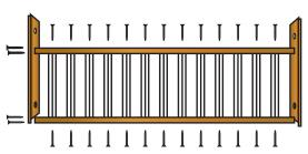
(5/4 X 5/4") SPINDLE (2 X 3") RAIL (5/4 X 4") FRET FRAME #10 X 2" SCREWS
