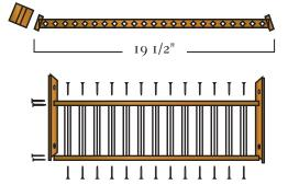
(5/4 X 5/4") SPINDLE (2 X 3") RAIL (5/4 X 4") FRET FRAME #10 X 2" SCREWS
