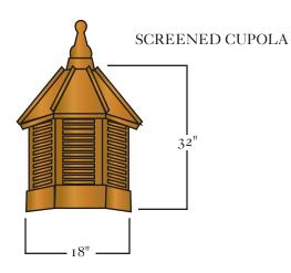
THE CUPOLA IS CONNECTED WITH STAINLESS STEEL SCREW FROM THE UNDER SIDE OF THE ROOF LATH.
