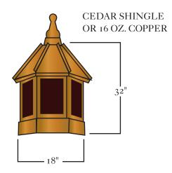
THE CUPOLA IS CONNECTED WITH STAINLESS STEEL SCREW FROM THE UNDER SIDE OF THE ROOF LATH.
